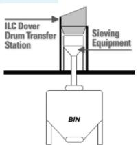
In the application pictured in Figure 3, powder is processed from a drum, through a mill (a Quadro Sifter in this example), into a stainless steel Intermediate Bulk Container (IBC).
